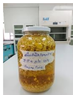
Step 4: Soak the pomelo peel in the solvent. Use 250 g of pomelo peel/750 ml of ethanol.
