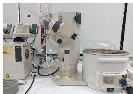
Step 6 Evaporate the obtained solution to remove the solvent using a Rotary Evaporator.
