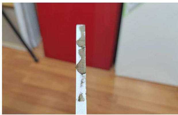
Figure 2: Matrix Stabilization via the Application of Lacquer Putty on the Flank Surfaces.
