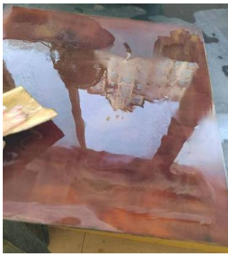
Figure 3: Sophisticated Abrasion of the EVA Matrix Substrate. Picture Source: Captured by the author.
