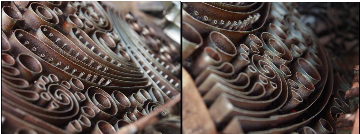
Figure2 :batik pattern stamps from used condensed milk cans
