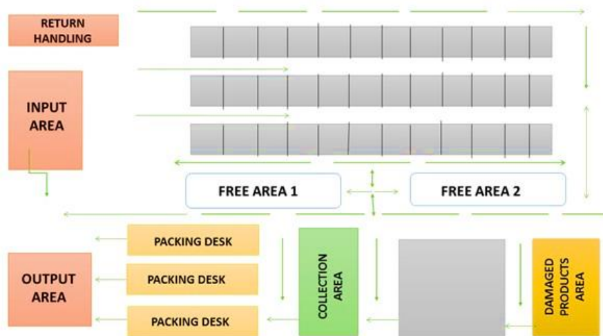
Figure 19. Example of the shop plan in the form of Mini or Micro-Fulfillment Center
