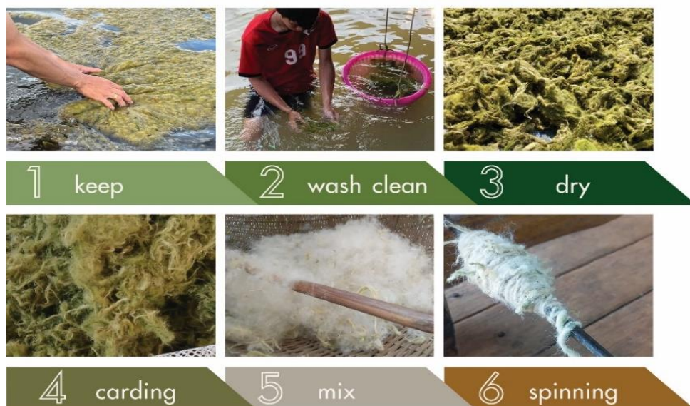
Figure 4 shows the preparation of algae for use. Source: Picture by researcher, Mongkol Ingkuthanon
