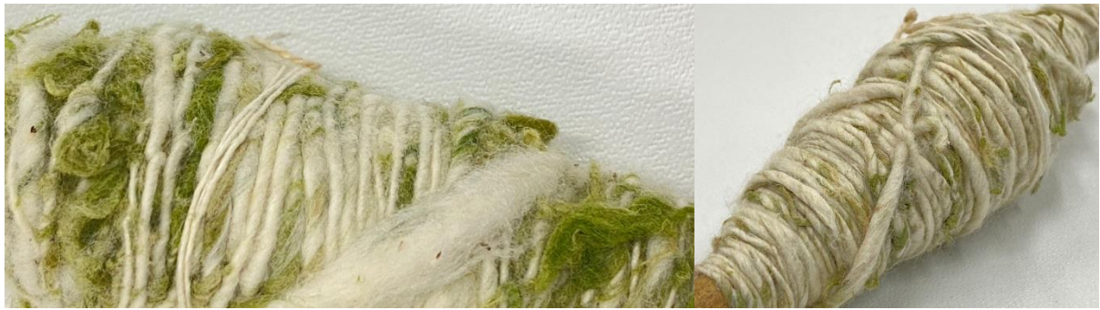
Figure 5 shows the algae fibers spun with cotton Source: Picture by researcher, Mongkol Ingkuthanon
