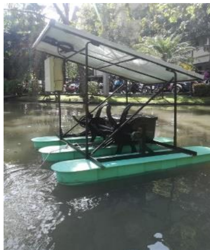
Fig.15. DC motor and reduction gear installation
