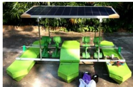
Fig.10. 3-buoy water machine driven by the photovoltaic energy system
