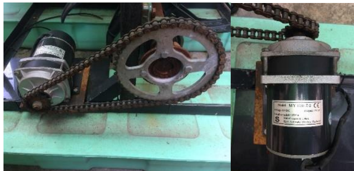
Fig.15. DC motor and reduction gear installation
