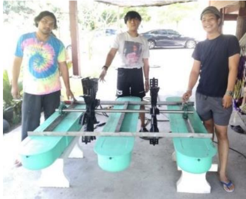
Fig.14. Paddle wheel installation on the floats
