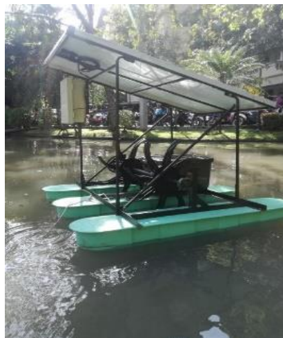
Fig.15. DC motor and reduction gear installation
