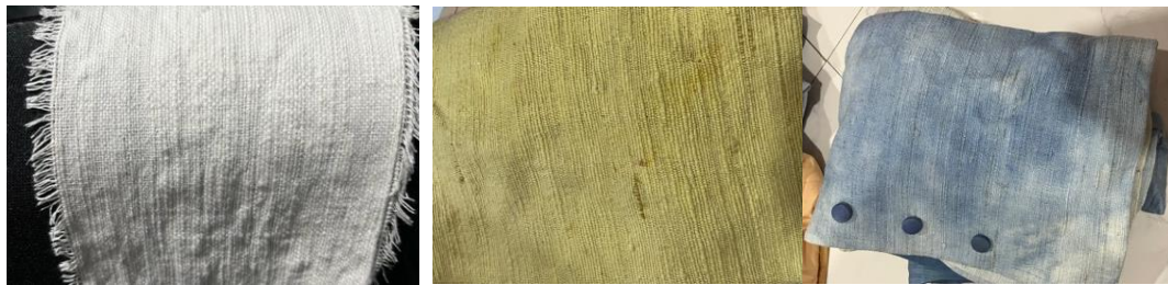
Figure 1: woven fabric of the Napier grass fibers Source: Siratcha Samleethong
