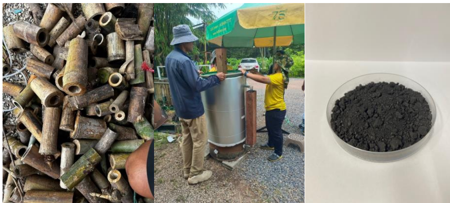
Figure 1: (left) Waste bamboo scraps, (middle) conventional furnace at bamboo garden in Rayong province and (right) bamboo biochar
